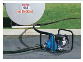
Gorman-Rupp portable Shield-A-Spark self-priming centrifugal pumps are the safest approach to handling flammable liquids with an engine-driven pump. The unit features a shielded ignition wire which provides an enclosed path for the high tension spark. The ignition switch is safe and spark-free, and the muffler is designed to retard sparks.
